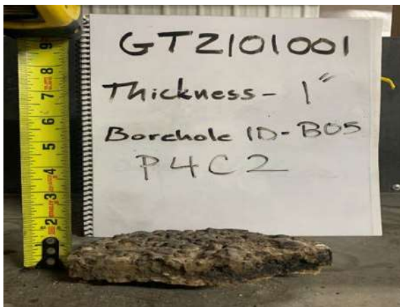
P4C2 B-5 - 1 in Asphalt Core
