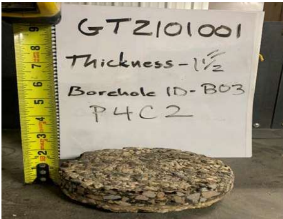
P4C2 B-3 - 1 1/2 in Asphalt Core
