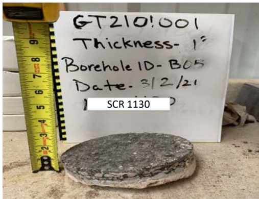
SCR 1130 B-5 - 1 in Asphalt Core
