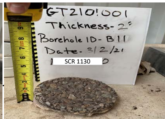
SCR 1130 B-11 - 2 in Asphalt Core
