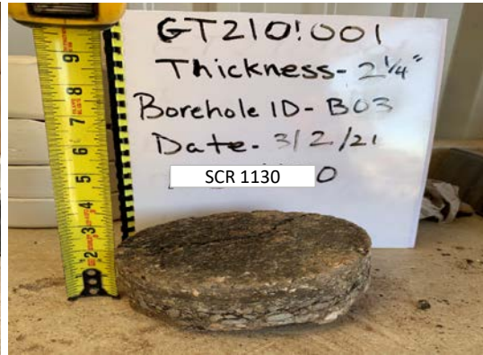
SCR 1130 B-3 - 2 1/4 in Asphalt Core
